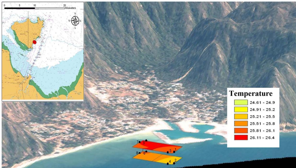
Figure 3: Study site at Nelly Bay, Magnetic Island, Australia. The sensor network consisted of 4 moorings (1-2, 3-4, 5-6 and 7-8). Each mooring has 7 sensors deployed on vertical scale 2 meters apart and 2 data loggers (Figure 2). Each data logger has a number on the map 1-8. The temperature surfaces were extrapolated from the data loggers point data recorded on 17/09/07 (for the illustration purpose only).
