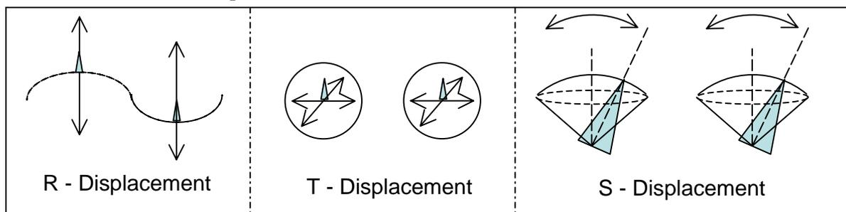
Figure 3: First order displacement on a buoy. Three basic displacements caused by wave motion.
