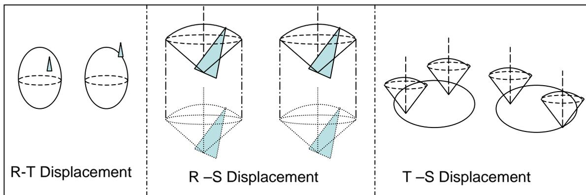
Figure 4: Second order displacement of a buoy.
