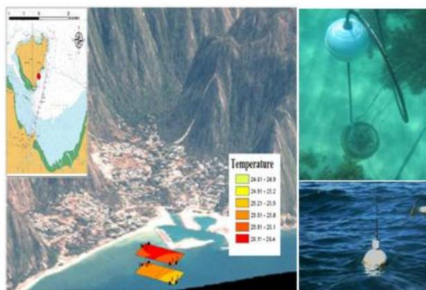
Figure 2: Sensor nodes used in deployment in Nelly Bay, Magnetic Island, GBR Australia [13].
