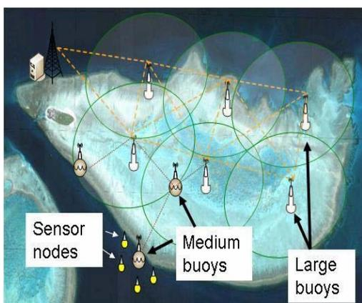
Figure 1: Sensor network schematic for planned deployment in Heron Island, GBR Australia
