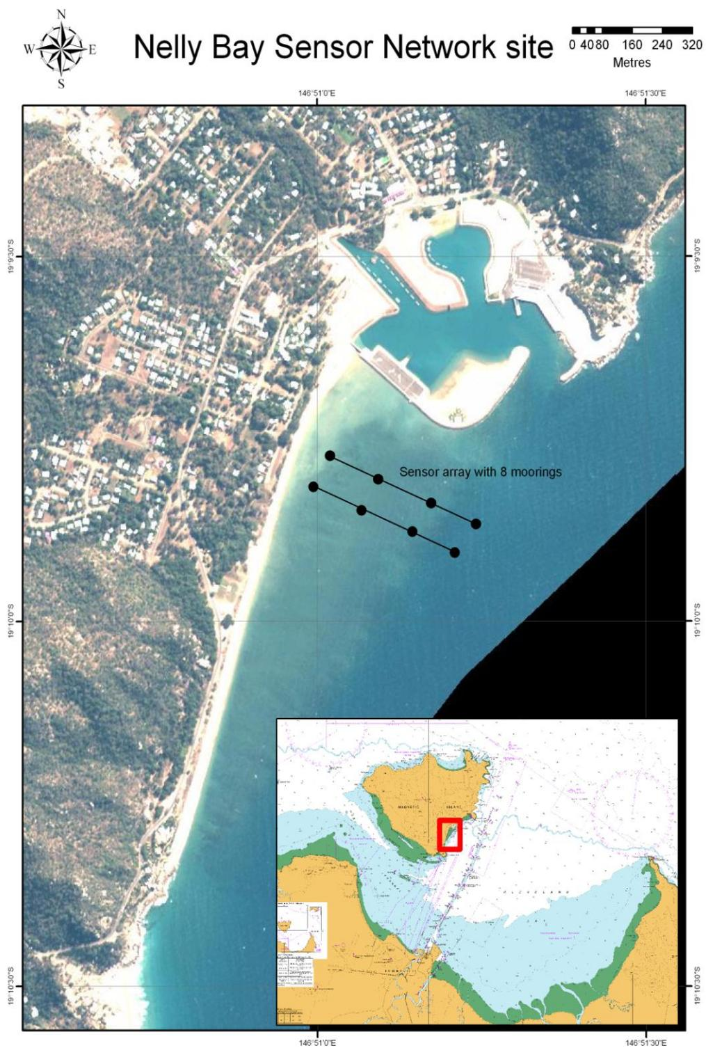
**Figure 6.** Study site at Nelly Bay, Magnetic Island, Australia. The sensor network consists of 2 transects with 4 moorings per array. Each mooring has 7 sensors deployed on vertical scale 2 meters apart (Fig. 5)
