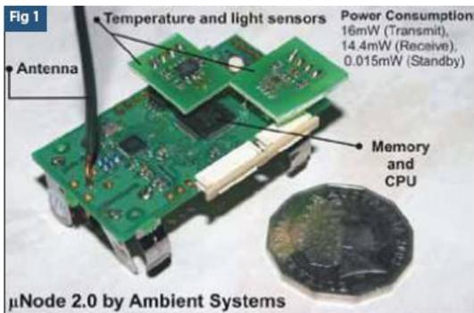
**Figure 3.** Unode supplied by Ambient Systems | 19 |
