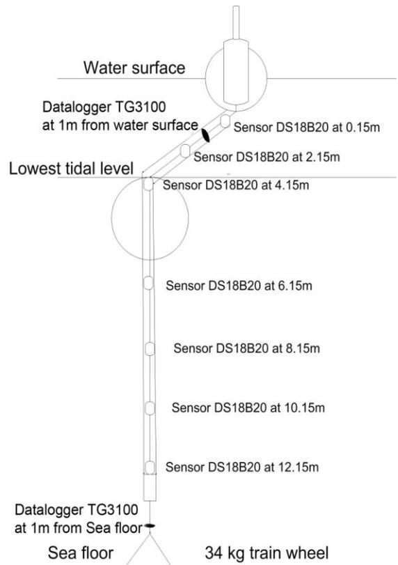
**Figure 5.** Diagram of the sensor buoy with seven DS18B20 digital thermistors and TG3100 dataloggers.
