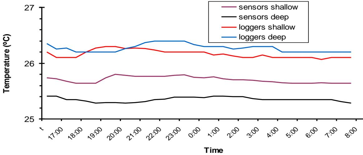
**Figure 8:** Temperature data collected by the data loggers (TG3100) and real time sensors (DS18B20) at the outer mooring station of transect 2 on 21<sup>st</sup> and 22<sup>nd</sup> of September 2007. The data loggers and real time sensors were fixed on the same mooring line at two depth levels: shallow (within 1 meter from the surface) and deep (1 meter from the sea floor).
