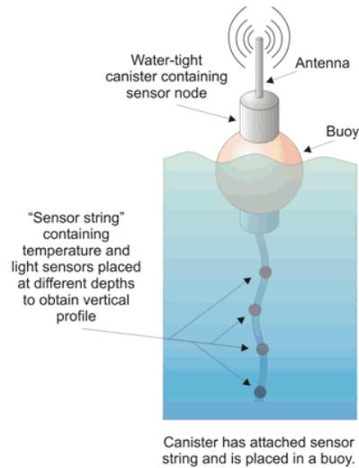
**Figure 4.** Sensor string design showing the position of underwater temperature sensors and RF transmitter attached to the buoy | 19 |
