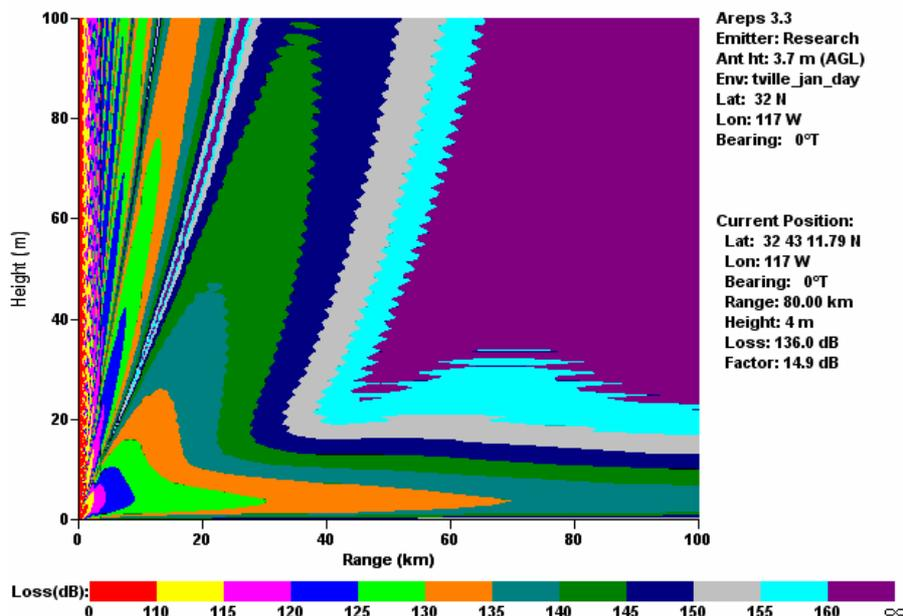
Figure 3. Transmission propagation for 10.4 Ghz microwave link showing how the waves at low height are able to travel long distances with acceptable loss.
