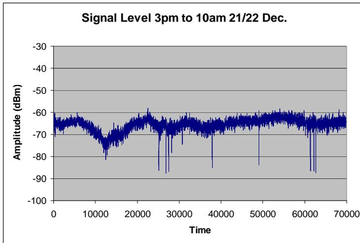
Figure 4 . Received signal Amplitude of IF signal versus time.
