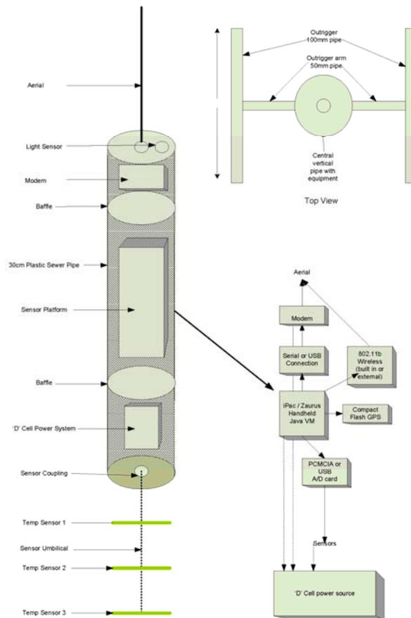
Figure 4. Schematic of a possible sensor design
