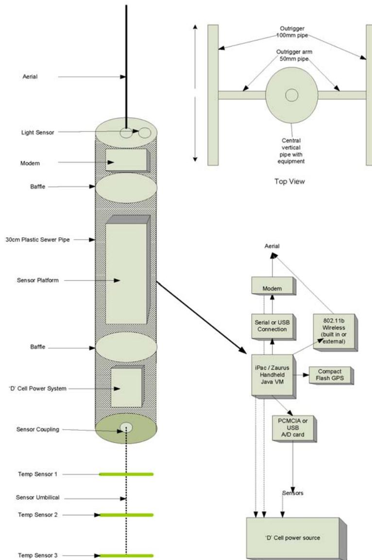
Figure 3. Draft sensor design
