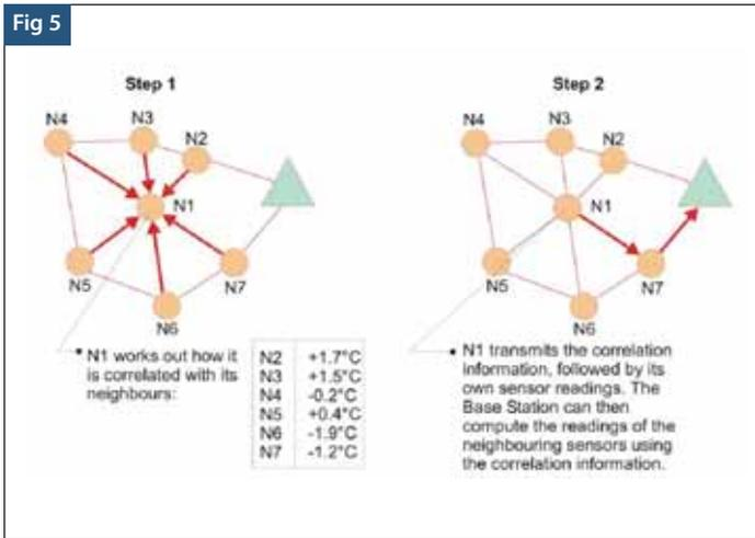
Reducing the amount of data that needs to be transmitted by taking advantage of spatial correlations of sensor readings.
